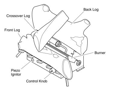
Figure 2 - Vent-Free Gas Log Heater - Single Burner (Mountain Oak Logs Shown)
